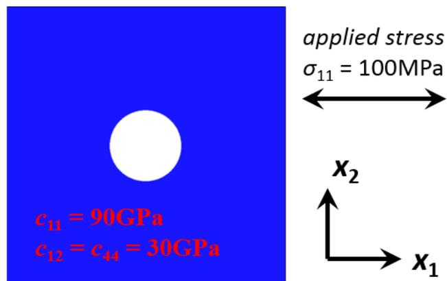
**Figure 5.2.1** Schematics of the example of stress concentration in solid-gas system.
