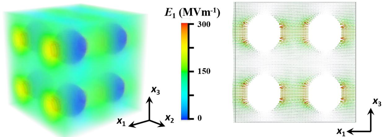
**Figure 5.3.2** Electric field distribution on applying an external electric field  $E_1 = 100 \text{ MV/m}$ . (Left) heat plot of  $E_1$ ; (right) vector plot of  $E$  in the cross-section through the center of the dielectric particles.
