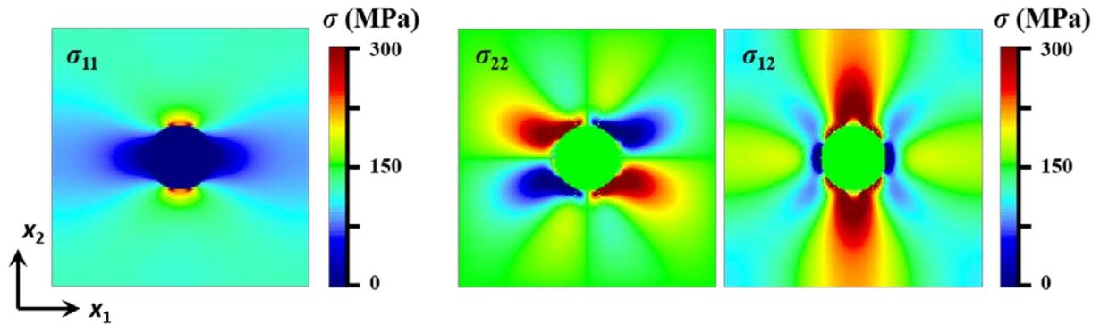
**Figure 5.2.2** Stress distribution on applying an external stress  $\sigma_{11} = 100\text{MPa}$ .
