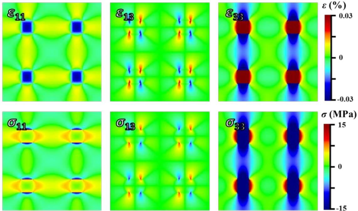
**Figure 5.4.2** Spatial distribution of strain and stress on applying an external electric field of  $E_3 = 20$  MV/m.
