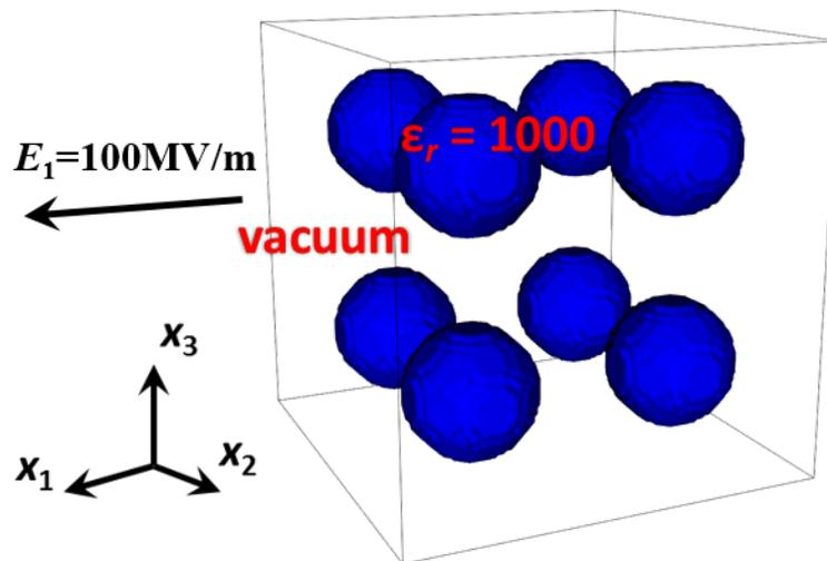
**Figure 5.3.1** Schematics of the example of dielectric particles in vacuum.
