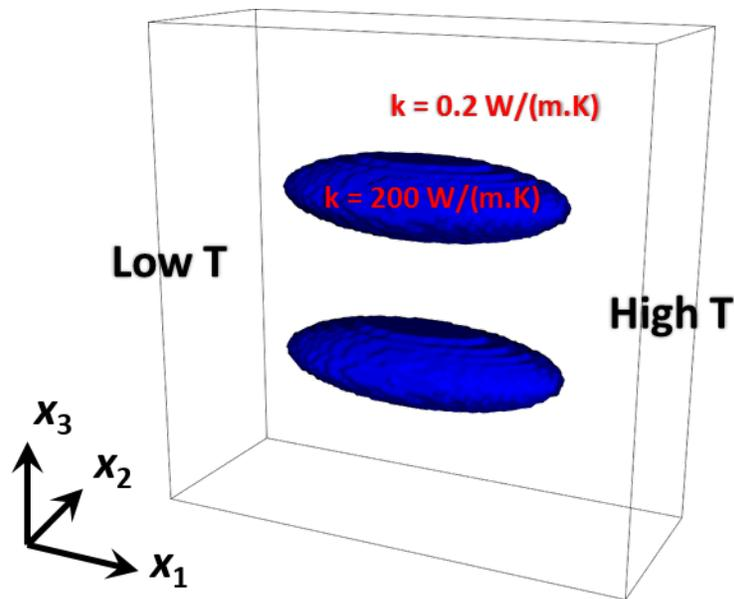
**Figure 5.1.1** Schematics of the example of thermal conduction in a matrix-inclusion system.
